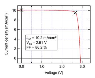
Fig. 9. Light J-V curve of the IMM-3J device under 1-sun irradiance calibrated AM1.5 global spectrum (1000  $W/m^2$ ). The device does not have anti-reflective coating.
