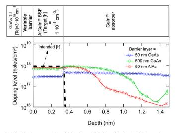
**Fig. 3.** Hole concentration [h] depth profile along the phosphide layers of test structures that mimic the GaInP top subcell of an IMM-3J with a [Te] =  $3 \cdot 10^{19}$  cm<sup>-3</sup> in the GaAs cathode using several barriers: 50 nm GaAs, 500 nm GaAs and 50 nm AlAs. An ex-situ MOVPE bake at 675 °C for 60 min is performed in all samples to emulate the growth of a multijunction structure.
