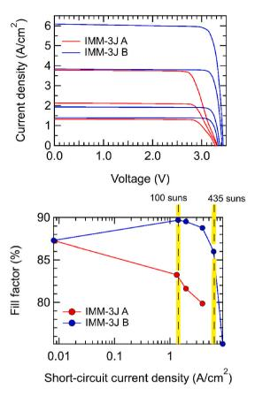
**Fig. 5.** Comparison of the concentration response of IMM-3J A and IMM-3J B devices with notable differences in the top cell R<sub>she</sub> (1230  $\Omega$ /sq and 300  $\Omega$ /sq, respectively) caused by Zn diffusion. Top: Light J-V at different irradiances. Bottom: Evolution of the fill factor at different short circuit current levels. The short-circuit current densities corresponding to 100 and 435 suns are indicated (considering J<sub>sc</sub>(1x) = 14 mA/cm<sup>2</sup>).
