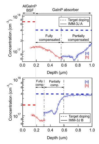
Fig. 4. Doping profiles along the AlGaInP/GaInP layers of the GaInP RHJ subcell of two IMM-3J designs using different target [Zn] in the BSF:  $7\cdot10^{17}$  cm<sup>-3</sup> in IMM-3J A (top) and  $2\cdot10^{17}$  cm<sup>-3</sup> in IMM-3J B (bottom).
