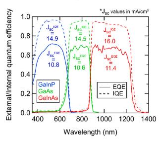
**Fig. 6.** External/Internal quantum efficiency of the individual subcells of the IMM-3J solar cell. The modelled collection efficiencies are 93%, 97% and 94% for the GaInP, GaAs and GaInAs subcells, respectively. The measured device does not have ARC. The values of the photocurrent densities ( $mA/cm^2$ ) calculated for the EQE and the IQE using the AM1.5 direct solar spectrum normalized to 1000 W/m<sup>2</sup> are included.
