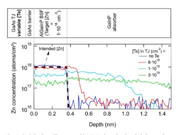
**Fig. 2.** [Zn] depth profile measured by SIMS along the phosphide layers of test structures that mimic the GaInP top subcell of an IMM-3J structure with variable [Te] in the GaAs cathode: no doping,  $8 \cdot 10^{18}$ ,  $1 \cdot 10^{19}$  and  $3 \cdot 10^{19}$  cm<sup>-3</sup>. An ex-situ MOVPE bake at 675 °C for 60 min is performed in all samples to reproduce the growth of a multijunction structure.
