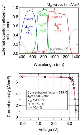
Fig. 10. Top: EQE and R of the IMM-3J with ARC, with indication of the  $J_{sc}$  for each subcell under the AM1.5 direct solar spectrum Bottom: Light J-V curve of the IMM-3J with ARC under 513-sun irradiance.
