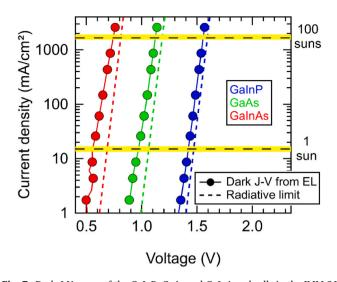
**Fig. 7.** Dark J-V curve of the GaInP, GaAs and GaInAs subcells in the IMM-3J obtained by using the EL technique. The modelled curves in the radiative limit are included (note that this modelling considers the effects of the internal optics in the management of internally emitted photons). The  $\eta_{ext}/\eta_{int}$  values obtained at 1 sun current densities are: 1.2/51.9%, 0.2/25.7% and 0.1/5.5% for the GaInP, GaAs and GaInAs subcells.
