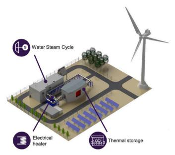
Fig. 3. Schematic of ETES system.
