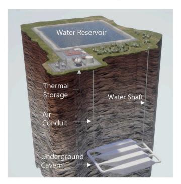
Fig. 2. Adiabatic CAES system developed by Hydrostor.
