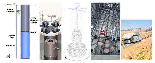
Fig. 1. a) illustrative plot of Gravity Power Module from Gravity Power Inc. [56]; b) Schematic plot of the Gravitricity system [53]; c) Design from Energy Vault [54]; d) Lifted Weight Storage module constructed by Energozapas [57] e) ARES's demonstration project in California [58].
