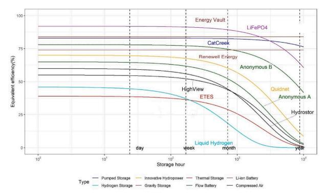
Fig. 5. Equivalent efficiency of different storage technologies as a function of time. Idle loss of LFP is based on [38] and does not include parasitic energy uses that may be highly dependent on operating conditions (e.g. air conditioning).
