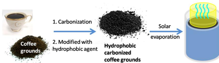
**Scheme 1.** Schematic of the process flow for the preparation of the HCCG.
