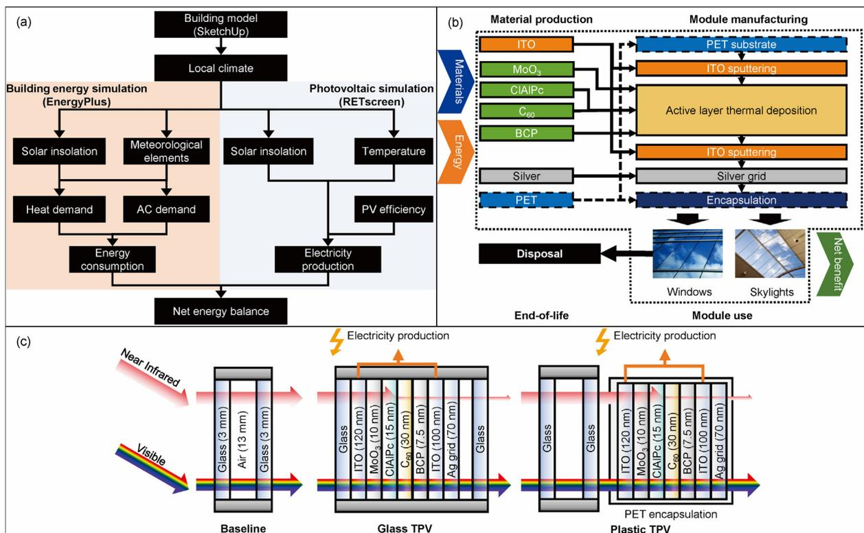
**Fig. 1.** (a) Overview of the modelling approach that combines the building and photovoltaic simulations to calculate the net energy balance, (b) LCA scope for transparent organic photovoltaic and (c) window architecture for the baseline double pane window and transparent photovoltaic either incorporated in the window structure (Glass-TPV) or externally using encapsulated TPV (Plastic-TPV).
