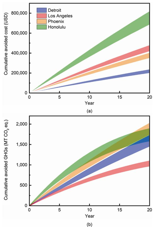
Fig. 8. Cumulative avoided (a) cost and (b) greenhouse gases over the 20 year lifetime of glass transparent PV window ( $\eta = 10\%$   $T_{50} = 25$  yrs), where the lowest value corresponds to application on the South, East and West (SEW) direction of the building and the highest with the addition of the North face (SEWN).
