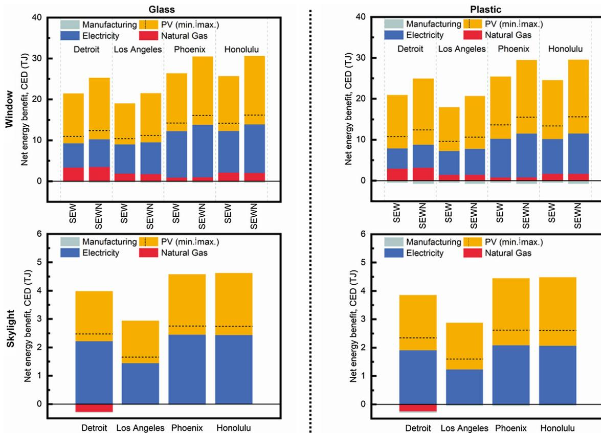
Fig. 6. Net cumulative energy benefit for glass and plastic TPV for window and skylight applications for all four locations. The photovoltaics electricity generation was based on the current (min:  $\eta = 3\%$ ,  $T_{50} = 7$  yrs) and future (max:  $\eta = 10\%$   $T_{50} = 25$  yrs) technologies.
