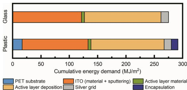
Fig. 5. Cradle to gate cumulative energy demand for the production of 1 m<sup>2</sup> Glass-TPV and Plastic-TPV modules.
