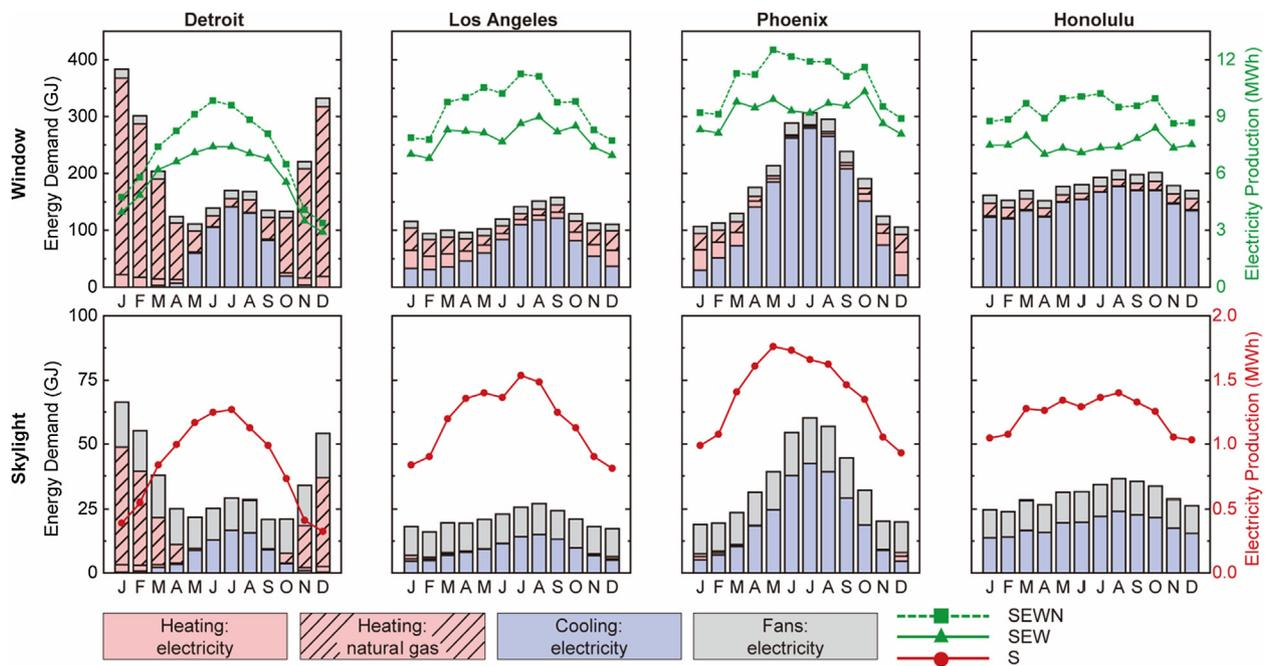
Fig. 4. Annual building energy demand and electricity production for a TPV ( $\eta = 10\%$ ) for the four cities considered with window replacement on the south east west-north (SEWN) or south-east-west (SEW) directions and for the skylight application.
