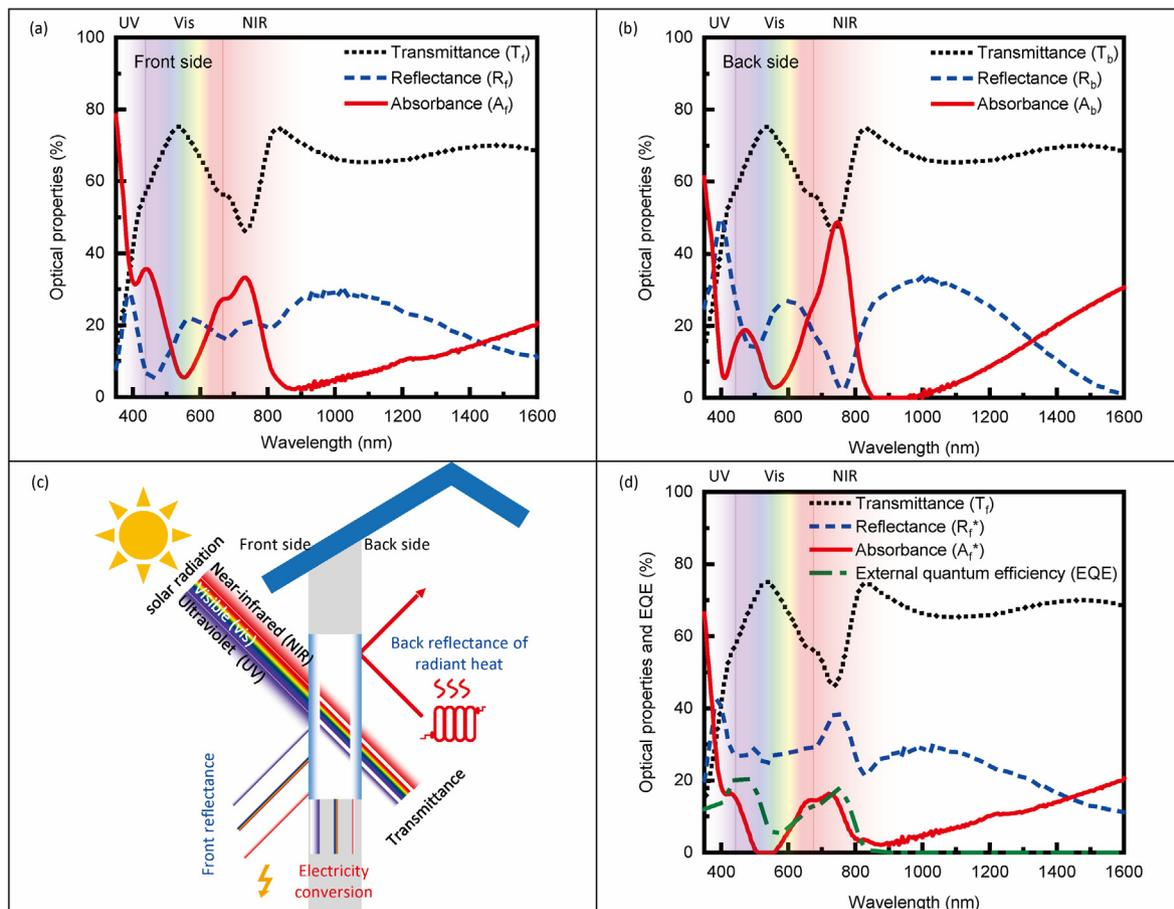
**Fig. 3.** Transparent photovoltaic UV-vis spectra for (a) front illumination and (b) back illumination. (c) The proportion of the solar radiation in range of ultraviolet, visible, and near-infrared for reflectance, transmittance, and electricity conversion and, (d) corrected front illumination absorbance and reflectance spectra used in the EnergyPlus simulation to account for the electricity generation.
