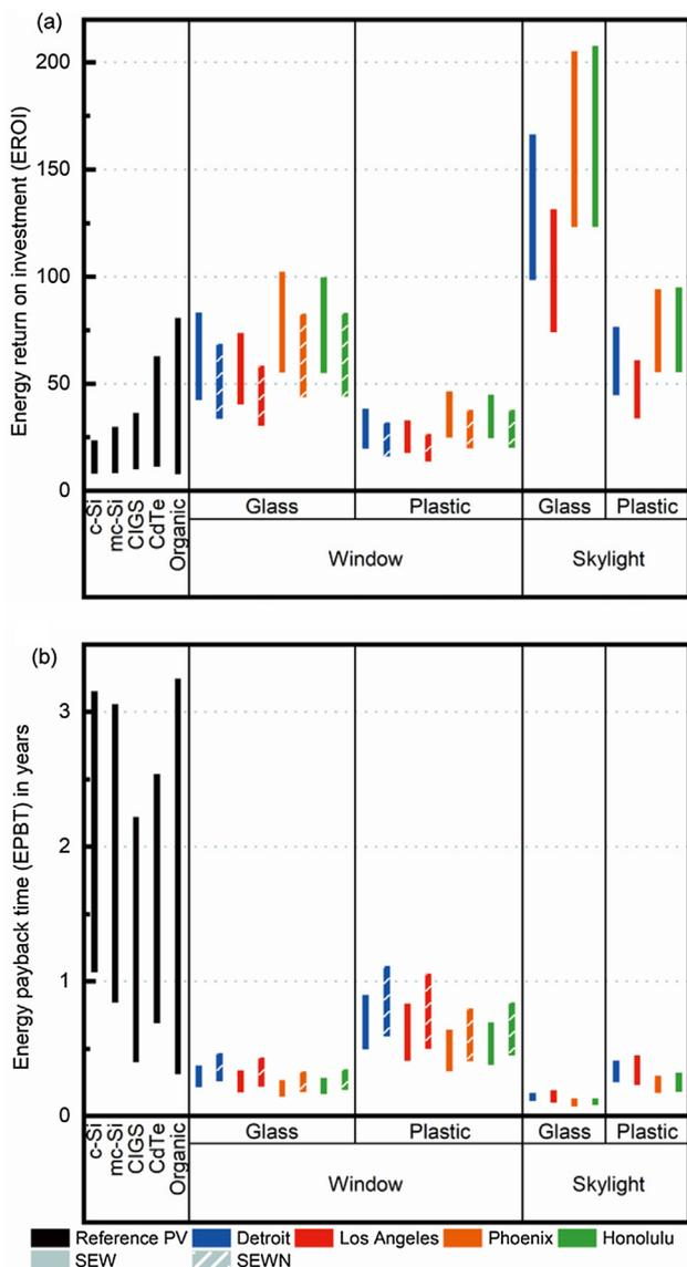
Fig. 7. (a) The energy return on investment (EROI) and (b) energy payback time (EPBT) for all types of transparent photovoltaics considered. For comparison purpose, the EROI and EPBT for various types of modules manufactured after 2009 were calculated under standard conditions (25 years lifetime and 1000 W/m<sup>2</sup> insolation) [58].
