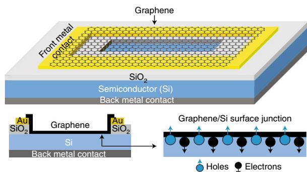
**Fig. 1 | Schematic of a graphene-on-semiconductor (Si) heterojunction photovoltaic cell.** Top: top view of the heterojunction. Bottom: side view of the heterojunction (left) and charge-carrier transport across the surface junction (right).
