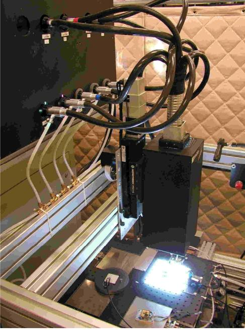
Fig. 2. Photograph of one-sun multisource solar simulator.
